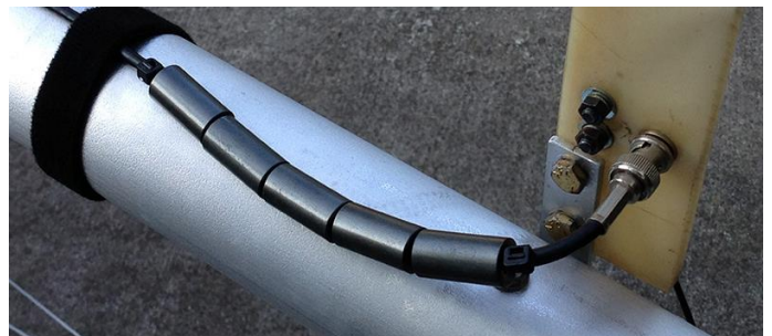
Figure 14 – Antenna mounted using an L-bracket. Anything similar will work as well.
