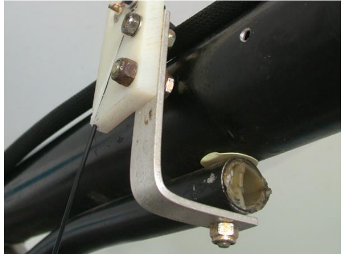
Figure 13 – Five ferrite cores secured with wire zip ties at antenna connector end of coax feed line.
