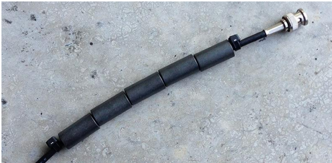
Figure 13 – Five ferrite cores secured with wire zip ties at antenna connector end of coax feed line.
