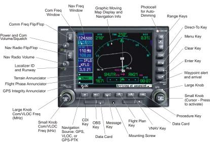
Figure 1 - 530W Series Control and Display Layout
