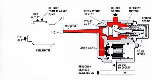
THERMOSTATIC BYPASS AND CHECK VALVE
