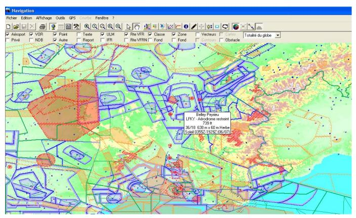
It interfaces well with all kinds of GPS navigators but one can also use FF Navigation itself on a (tablet) PC as onboard moving map. This is an interesting solution for the eVFR tests and demos as a (tablet or micro) PC is the best development and experimentation platform.
