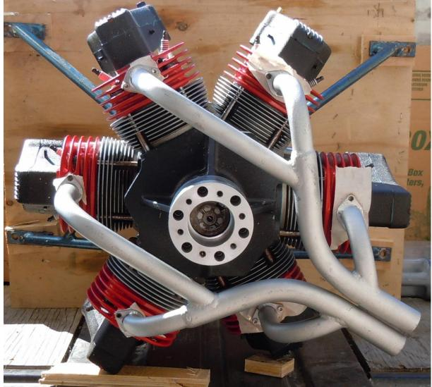
R1765 Sadler Radial Engine with capacity of 65 h.p. [71]
