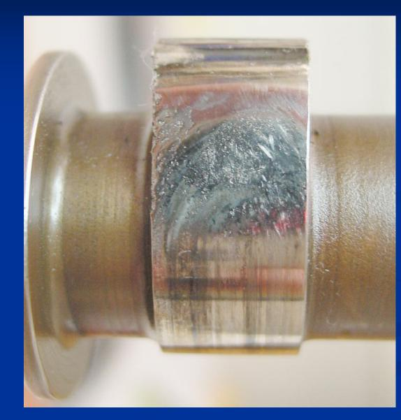
Pitting leads to catastrophic cam failure
