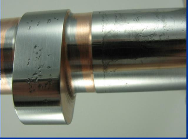
**Rust affects** all steel parts 300 Hours Not the solution to Lycoming cam problems
