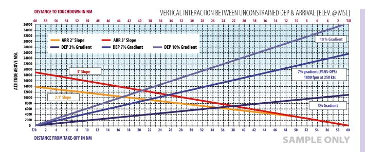
For example: if a departure on a 7% climb gradient (marked on graph) had travelled 25 track miles from the departure end of the runway (read on lower X axis) when it crossed the arrival on a 3° slope which was at 35 track miles from the runway (read on upper X axis), both aircraft would be in the region of 11,000 feet AMSL. So choosing this crossing point would not be efficient because it would restrict the departure's continuous climb and the arrival's continuous descent.
