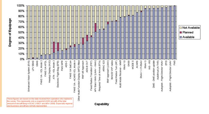
An equipage questionnaire culminating in a graph such as the one above (a 2010 European Avionics Survey) is a useful tool for analysing fleet capability
