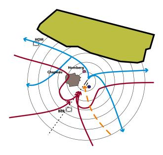
Key to obtaining these advantages (particularly in a terminal airspace) is the need for arrival and departure routes (STARs/ IAPs and SIDs) to be designed as a function of the interaction between them as well as servicing the traffic's desired track and ensuring obstacle clearance. Route placement for PBN does not negate best practices in route design developed over decades. Some of these are provided below.
