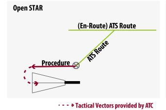
procedure will require tactical routeing instructions to align the aircraft with the final approach track. This results in the RNAV system only being able to calculate the descent up to the final waypoint on the procedure. This means that a continuous descent operation after this point may not be possible, due to the uncertainty of path stretching which ATC may use.
