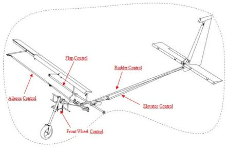
Figure 7-7 Flight control diagram
