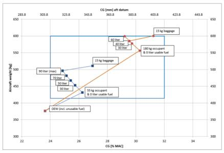
Figure 6-1 Approved weight and balance envelope
