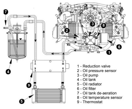
Figure 7-10 Lubrication system diagram
