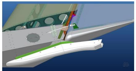
Figure 7-4 Draining system – tail skid aerodynamic fairing
