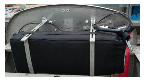
Figure 7-20 AEPS canopy container with packed chute
