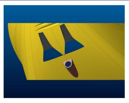
Figure 7-2 Draining system – lower engine cowling – hole between air inlets
