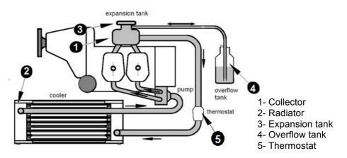
Figure 7-11 Cooling system diagram
