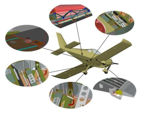
Figure 7-1 Draining system – fuselage
