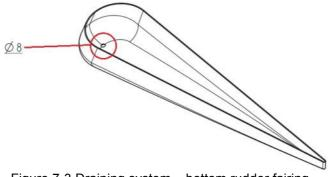
Figure 7-3 Draining system – bottom rudder fairing
