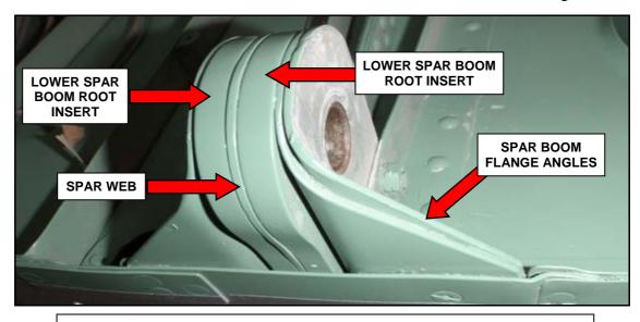
FIG. 6. CHIPMUNK WING LOWER SPAR BOOM SHOWING ROOT INSERTS
