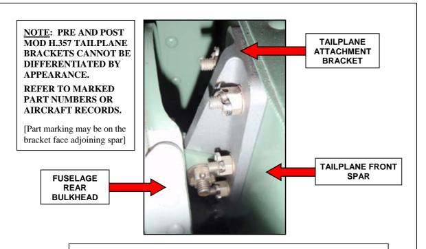
FIG. 9. TAILPLANE ATTACHMENT BRACKET (Port bracket illustrated)
