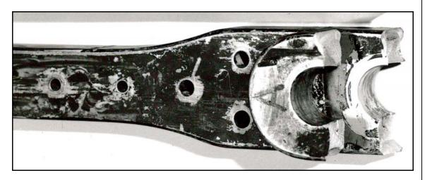
FIG. 2. FAILED LIGHT ALLOY FUSELAGE CENTRE SECTION TIE BAR
