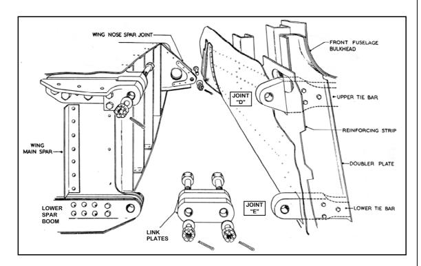
FIG. 1. CONFIGURATION OF WING-TO-FUSELAGE SPAR ATTACHMENTS
