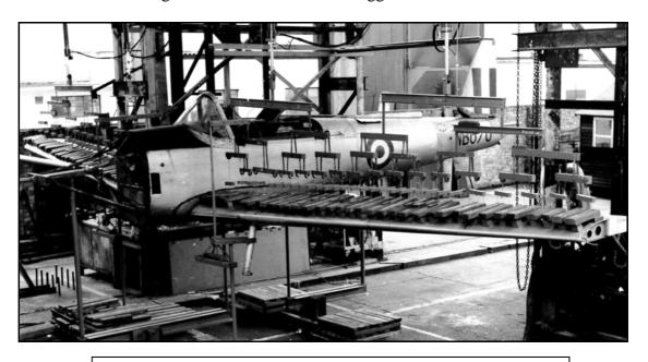
FIG. 3. DHC-1 CHIPMUNK T MK 10 - FULL-SCALE FATIGUE TEST
