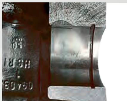
Fig. 3 Cross section of a piston pin boss
