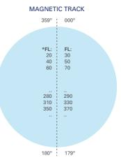
\*If below the transition altitude (see p.84), the levels should be flown as altitudes, such as 3500 ft, 4500 ft and so on.
