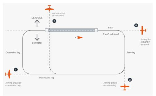
**Downwind join** involves directly joining the circuit parallel to the runway in the downwind direction. It is important to observe the direction of the crosswind leg, since that is where potentially conflicting circuit traffic will come from. If in doubt about cutting in front of another aircraft, slow down and/or manoeuvre to fit in behind.
