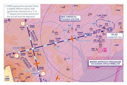
A typical RNAV (GNSS) approach established outside controlled airspace. In this case Exeter airport.
