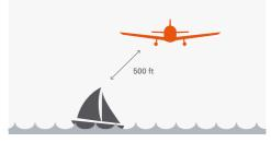
Note: <sup>1</sup>The standard rule under the European Rules of the Air for a VFR flight is to not to fly **below 500 ft above ground level**, unless taking off or landing. The UK has used the permitted national discretion, in order to provide a more flexible rule for aircraft flying in the UK. When flying in other European states the standard SERA rule may apply.
