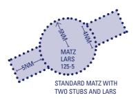
Aircraft operating near military aerodromes are not confined to the MATZ. This could include aircraft approaching to land or operating in what is known as the 'radar training circuit' (RTC). The RTC is a relatively standard pattern flown by aircraft around the aerodrome for the purpose of practising radar approaches.
