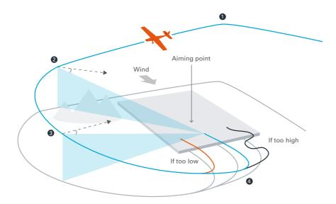
A commonly taught forced landing technique is that of the 'constant aspect'. The full pattern assumes a height of around 2000 ft or more, although the main principle of it applies at any height. Assuming you are sitting on the left, it is much easier to compete in a left hand direction.
