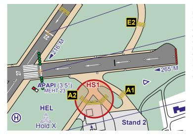
Holding points that are particularly vulnerable to runway incursion are marked on aerodrome charts as 'hot spots' and circled in red. The layout of taxiways at these points may be confusing and therefore pilots may be more prone to unintentionally entering the runway environment without clearance.
