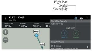
Flight Plan Loaded From Navigator
