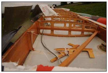
Photo No. 3: Damaged No. 2 rib with associated fragments.
