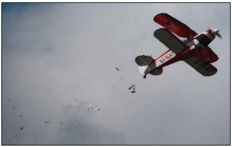
Photo No. 1: Sections of fabric separating from the upper wing (Peter Diffley)
