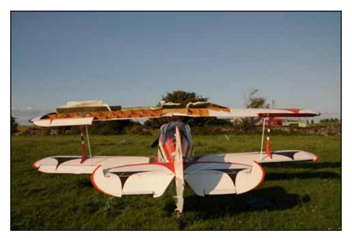
Photo No. 2: Fabric damage to the upper wing.
