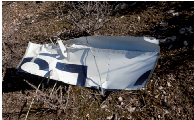
Fig. 3. Fragment from underside of left wing
